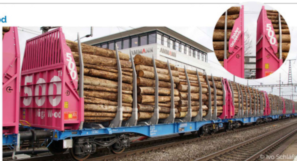
S657325 Innofreight articulated double timber transport wagon Sggmrrs | Innofreight Doppel Holztransportwagen Sggmrrs - A-IF 35 81 4657 325-0 "500TH Smart GigaWood"
