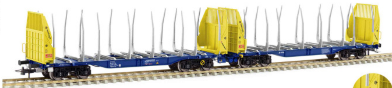
S657028 VTG articulated double timber transport wagon Sggmrrs | VTG Doppel Holztransportwagen Sggmrrs - D-VTG 37 80 4657 028-9 with SWISS KRONO AG logos | Mit SWISS KRONO AG Logos
